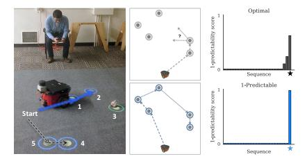
**Fig. 1.** Left: A participant controls the toy robot to clear the target that he believes will be third in the autonomous robot's sequence. Center: Schematic of the trajectory followed by the optimal (top) and 1-predictable (bottom) planner. Right: Predictability scores for each sequence under the optimal and 1-predictable planners after the robot has visited a single target. Here, optimizing for 1-predictability leaves a single high-score sequence, making it easier to identify.
